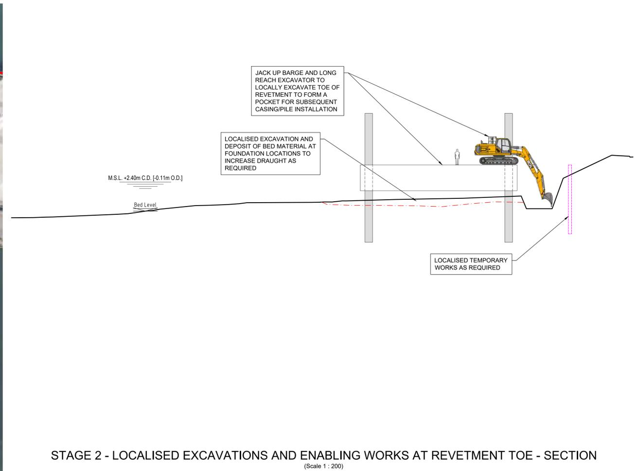
STAGE 2 - LOCALISED EXCAVATIONS AND ENABLING WORKS AT REVETMENT TOE - SECTION
